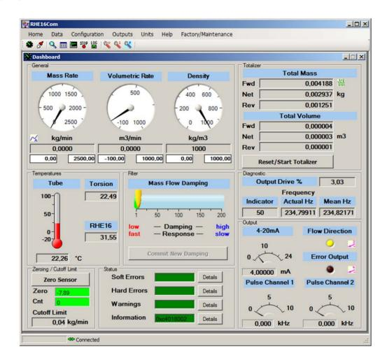
RHECom software is designed to ensure simple and expedient setup of the transmitter features and functions. The program operates on Windows<sup>TM</sup> based computers and has an intuitive user interface. Connection is via a standard USB port or the native RS485 connection of the transmitter. Communication between RHECom software and the transmitter uses MODBUS protocol.
