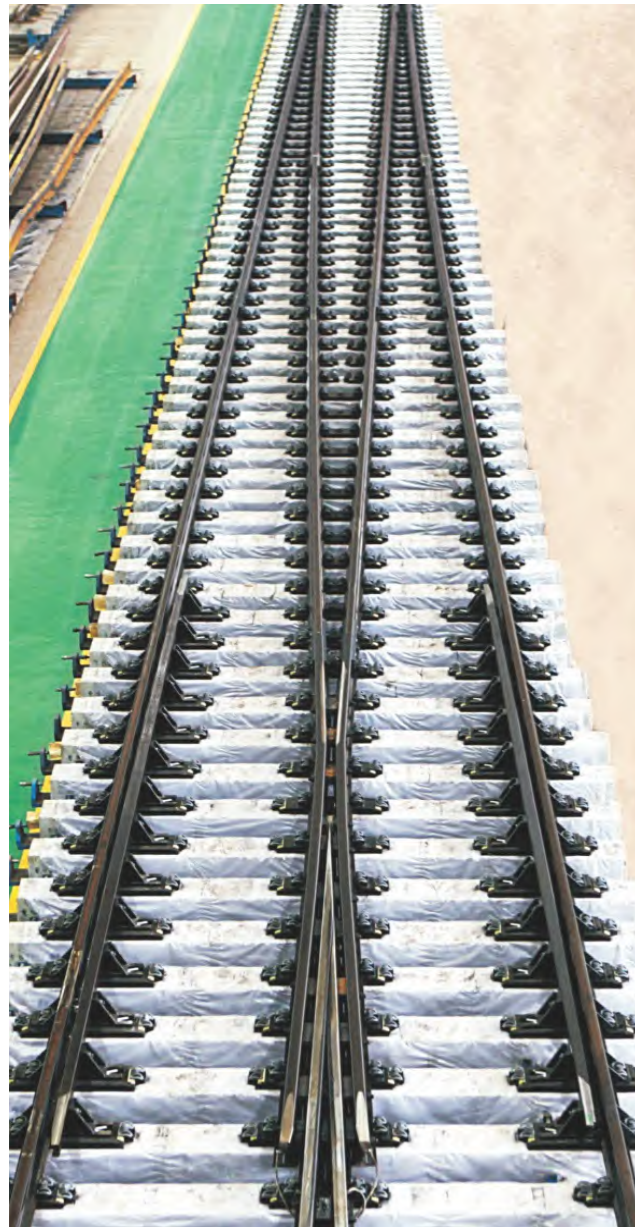
60kg/m Rail 1:18 Simple Turnout with Fixed Crossing for Heavy Haul Railway
