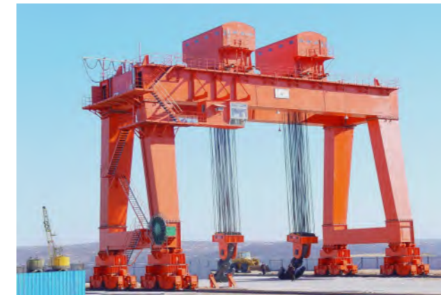
1100t double beam gantry crane
