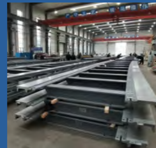
Manufacturing of maglev track panels
